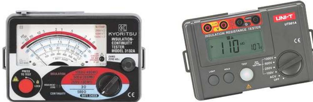
Insulation resistance test equipment.
