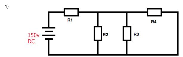
Refer to figure above is a series-parallel circuit, calculate the following values required. Given value R1=250 $\Omega$ , R2=380 $\Omega$ , R3=120 $\Omega$  and R4=320 $\Omega$ .
